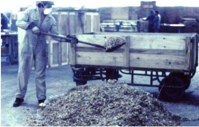
Figure 5.1. This worker is shoveling asbestos onto a cart. This is extremely dangerous and this worker has a high risk of dying from either lung disease or cancer as a result of this job. The dust mask he is wearing is not enough protection. He should be using a respirator that is designed for dangerous dusts and the material should be sprayed with water to keep dust levels down but, most importantly, asbestos should not be used at all, ever.
