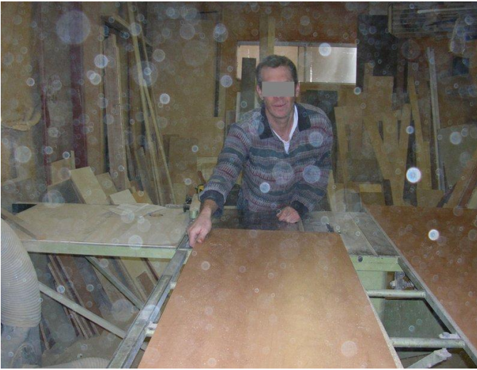
Figure 2.4. This worker is pushing a board into a table saw with his bare hands. See how close his arm is to the blade (on right). Also, you can see how dirty this workplace is by the dust on the lens of the camera. Workers here are breathing this dust all day. However, there is one good thing in this picture: the tubing on the left shows that there is a local exhaust system under the table that removes sawdust from under the saw. It is hard to know how effective the dust collection system is in this situation because there is so much dust around. (Photo courtesy of Seifeddin Ballal, University of Dammam.)
