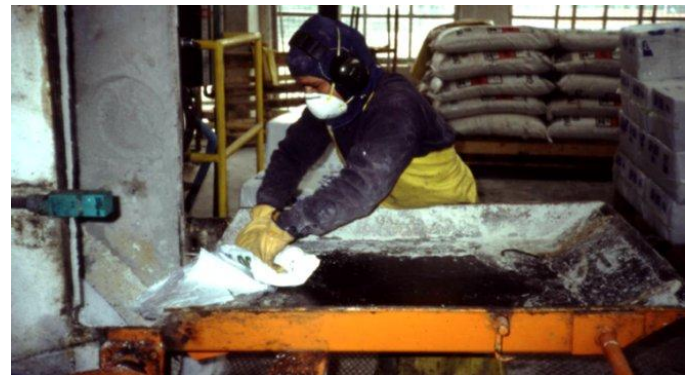
Figure 5.3. This worker is feeding asbestos into a chute where it will go to a vat to be mixed with cement. This is very dangerous work and puts the worker at risk of death from cancer or lung disease. The dust mask he is using is not effective against asbestos dust, so he and his supervisors only think that he is being protected when really he is not. Asbestos should never be used, ever. (Photo by Fernanda Giannasi, supplied with permission courtesy of René Mendes, Federal University of Minas Gerais – retired, Brazil.)
