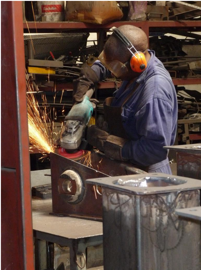
Figure 6.4. This worker in Nairobi, Kenya, is wearing three types of personal protective equipment: gloves, muff-type hearing protection, and goggle-type eye protection. This is the way it should be. The work of grinding metal parts can cause serious hand injuries, the noise can cause loss of hearing, and the flying particles of metal can severely injure the eyes, so all three are needed. (Photo courtesy of Suvi Lehtinen, Finnish Institute of Occupational Health.)
