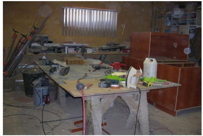
Figure 2.5. A cluttered, unsafe workplace. See the trip hazards on the floor, the unstable work surface (held down by bricks but supporting a hot iron), the long clamps against the wall that can fall down easily, poor lighting, several fire hazards, and dust everywhere (visible on lens of camera). (Photo courtesy of Seifeddin Ballal, University of Dammam.)
