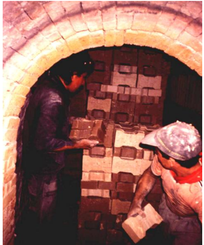
Figure 3.1. These workers are stacking unfinished bricks inside a kiln for firing. See how awkward it is to carry the bricks in one at a time. The workers use a cart on wheels to bring the bricks to the kiln area but the cart is too big to come closer. The man doing the stacking has to bend his head over to fit and needs to come out every few minutes to straighten his neck. These workers are also at risk for silicosis (see Chapter 5) because special bricks with a high silica content that can stand the heat, called “refractory” or “furnace” bricks are used in kilns or furnaces and repairing them is a dusty job. (Photo by Carlos Julio, supplied courtesy of Julieta Rodríguez-Guzman, Universidad El Bosque.)
